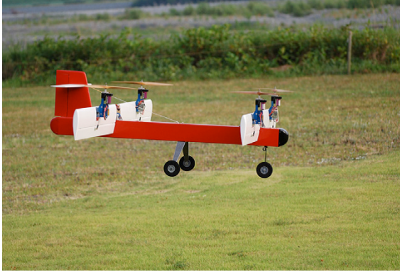
Figure 1.13: A quad-rotor design using an aerodynamic tail [16].
