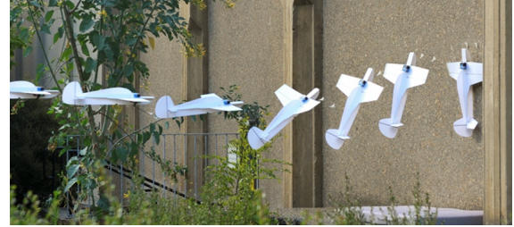
Figure 1.7: The Stanford perching UAV transitioning to vertical flight [9] .
