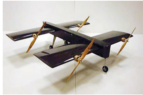
Figure 1.14: A quad-rotor design without stabilizing tail[17].
