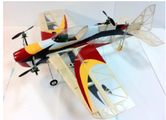
Figure 1.12: A modified RC plane for tri-rotor configuration [12].
