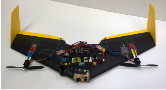
Figure 1.6: A top view of a tail sitter conceptual design[8].
