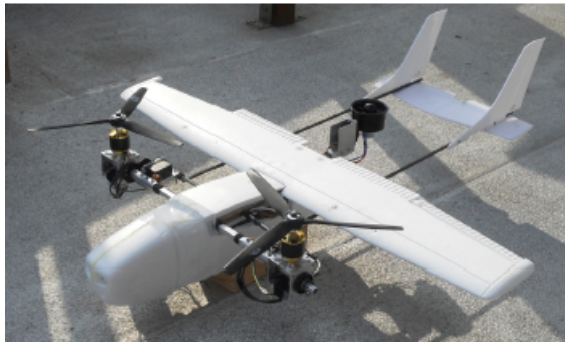
Figure 1.11: A tri-rotor with propellers off applied forward of the wing [13].
