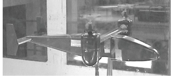
Figure 1.9: A manufactured dual propeller device undergoing wind tunnel testing [11].
