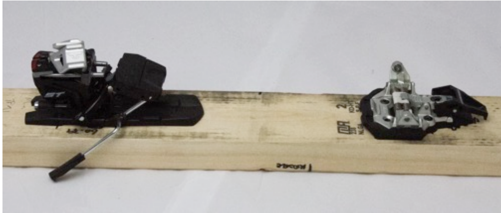
Figure 9.9: The Dynafit Radical ST used for testing as an exemplar AT binding. Indicator setting range: 4-10.
