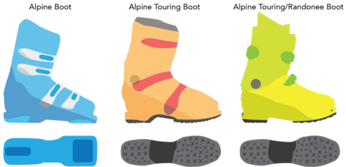
Figure 1.10: Alpine boots (left) differ from AT boots (center). AT/Randonee boots (right) are similar to AT boots and have metal inserts molded into the toe and heel to interface with Tech/Pin bindings.
