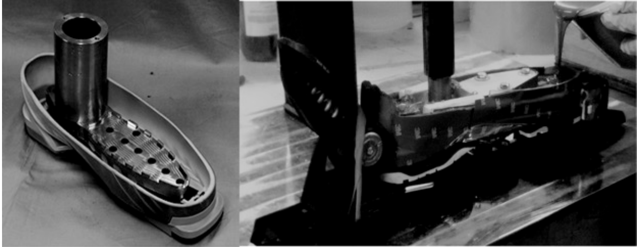
Figure 2.3: Preparation of ski boots for testing. Preparation of test boot soles required a metal adapter plate (left) to be fixed inside a cut boot shell using tooling compound (right). A custom jig was used to maintain proper alignment of the adapter plate-load cell interface relative to the boot.
