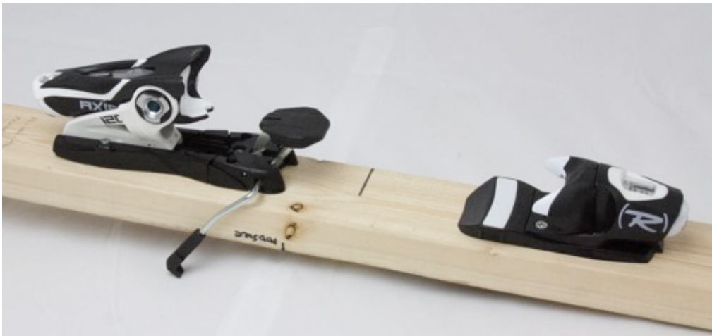
Figure 9.8: The Rossignol Axial 3 used for testing as an exemplar Alpine Binding. Indicator setting range: 3.5-10.
