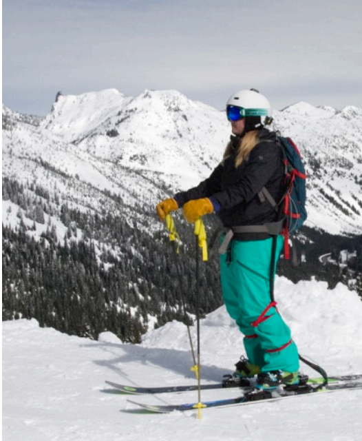
Figure 9.15: A female subject on skis with force plates mounted under the bindings. The cable from the ski extends to the backpack where the data acquisition unit and other electronics were housed. The XSENS MVN Biomech suit is under the subject's outerwear.
