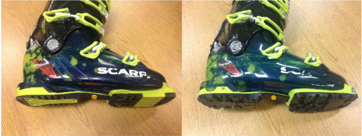
Figure 9.7: Alpine boot sole (left) and AT Boot sole (right) attached to the same boot shell model.
