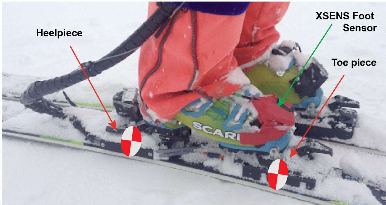
Figure 9.11: Two six-axis force transducers mounted under the toe and heelpieces of an AT ski binding. The XSENS IMU for each boot can be seen on the boot toe.
