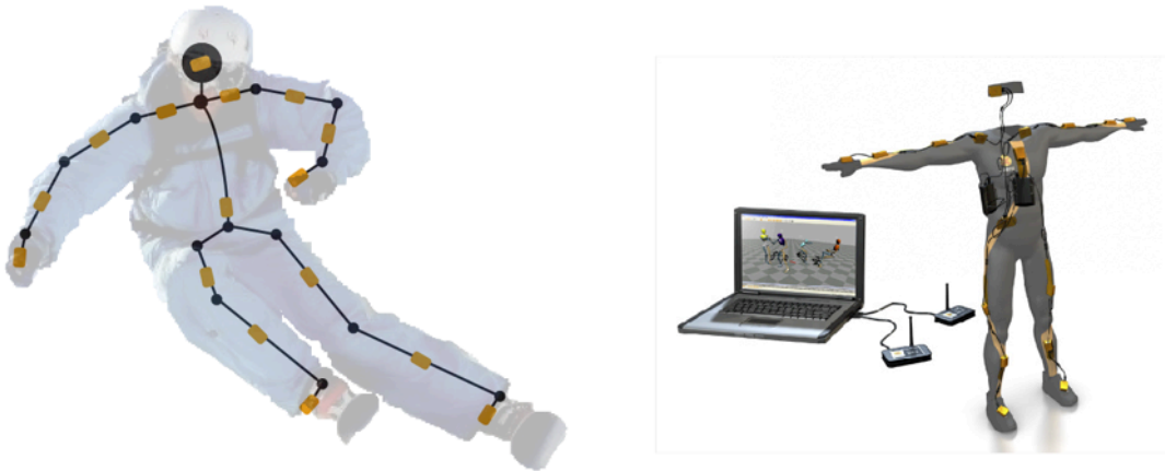
Figure 8.7: The XSENS MVN Suit allows for 3D kinematics to be measured on skiers outside of a laboratory systems with optical based systems.
