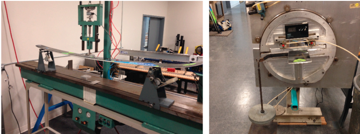
Figure 9.4: The flexural (left) and torsional (right) spring constants of each ski were measured per ASTM F779-12 and ASTM F489-12.
