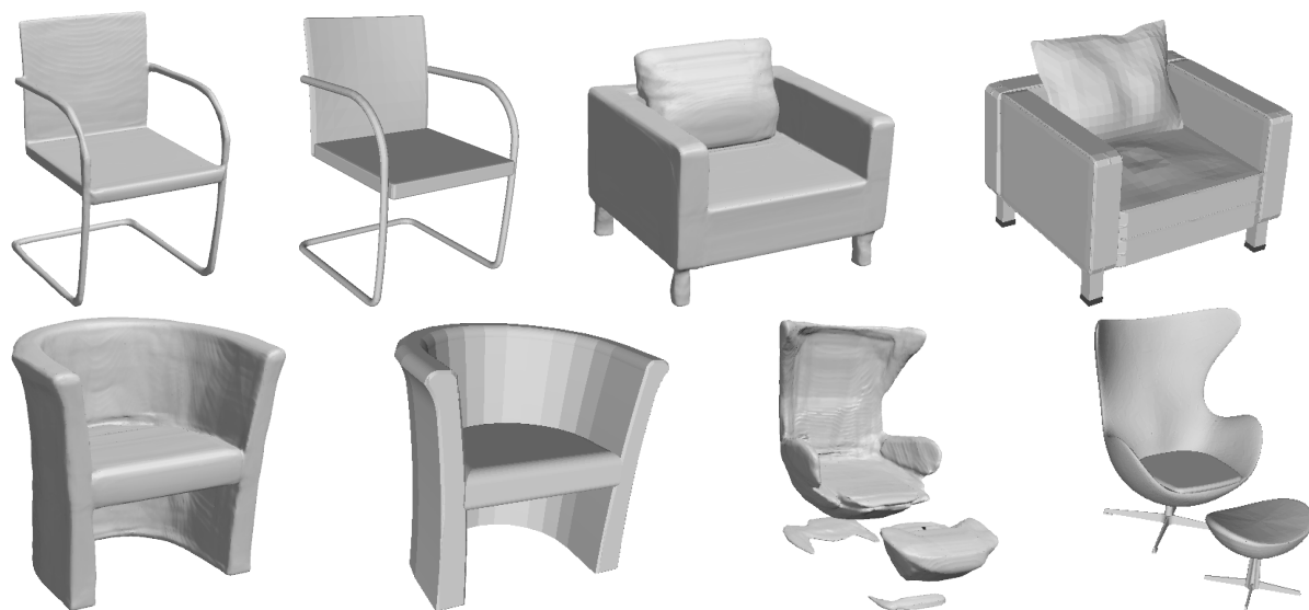
Figure 5.11: Additional test shape reconstruction results. Left to right alternatingly: DeepSDF reconstruction and ground truth.
