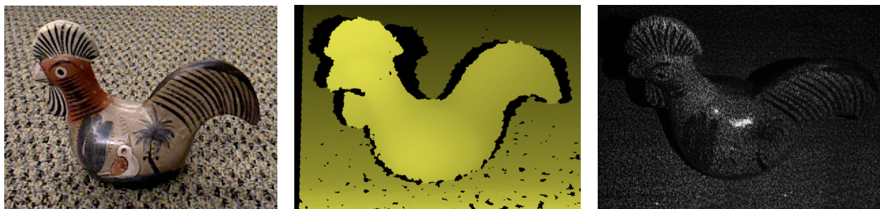
Figure 1.1: RGB-D input video streams to the system [184]. From left to right: sample RGB image, depth map image, infrared channel image. The system recovers surface specular property from the infrared laser system of the RGB-D camera.
