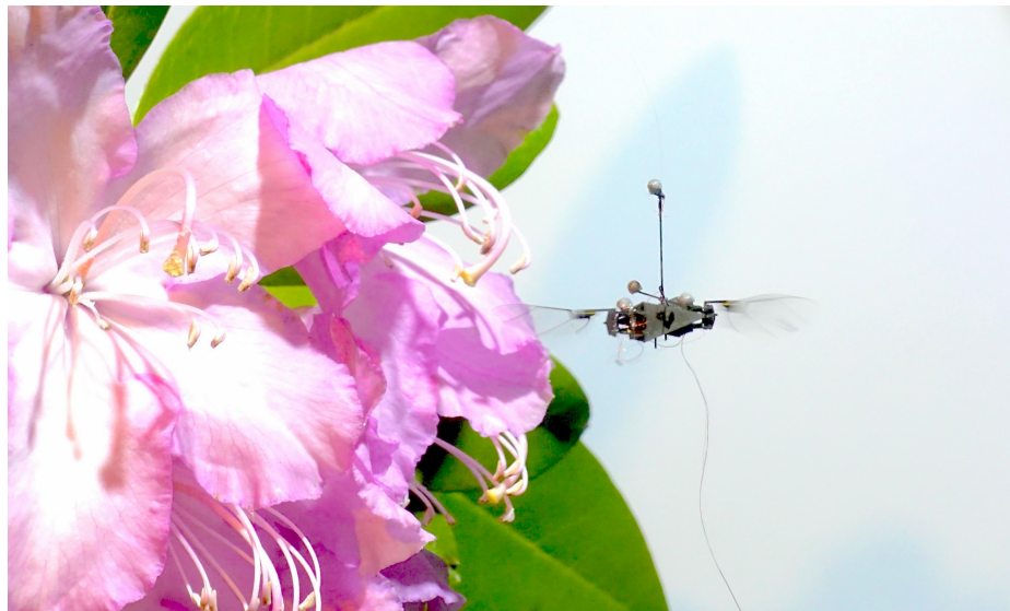
Figure 5.1: RoboFly, an insect-sized flapping robot weighing 146 milligrams, hovers next to a flower using feedback from motion capture cameras. The robot performs this hovering maneuver using the LQR controller reported in this work.
