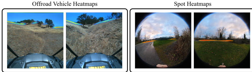
Figure 4.4: Example Heatmaps computed by LRN. The two images on the left show examples from the Racer Heavy. Blue is lower confidence and red is high confidence. LRN finds affordable spots between trees and on hill crests. On the Spot dataset on the right LRN correctly puts high score on the two forks in the road and to the side of bushes. For more qualitative results see Section 4.6.4.
