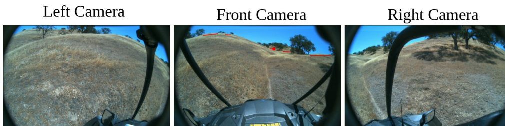
Figure 4.3: Labeling tool for affordance maps. The red lines in the center image are labeled affordable frontiers. Side images are for additional context but do not get labelled.
