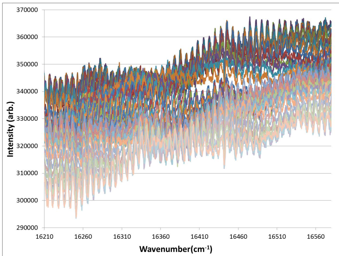
Figure 3-14 – Raw output using 2400g/mm grating for samples of 40 incremental RI steps.
