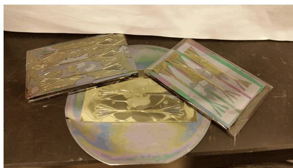
Figure 3.6: Thick layers of SU-8 caused significant film stress, resulting in delamination from the wafer during plasma treatment or during the hard bake step.
