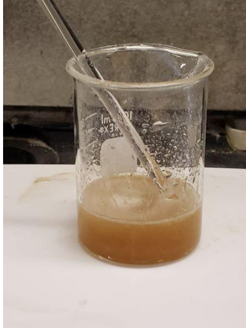
Figure 20. Alpha cellulose powder during acid hydrolysis with sulfuric acid.
