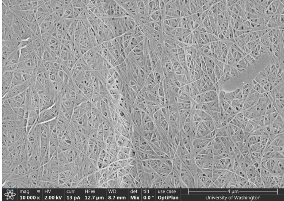
Figure 34. (BC41) SEM images of BC pellicles showing the individual nanofibers.
