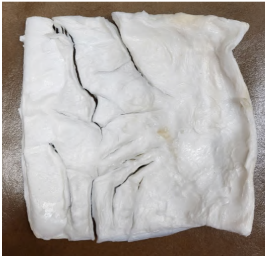
Figure 58. A 8 cm x 8 cm piece of liquid nitrogen frozen and freeze dried BC. Note the cracks that appear through the surface, causing issues with regular vacuum infiltration.
