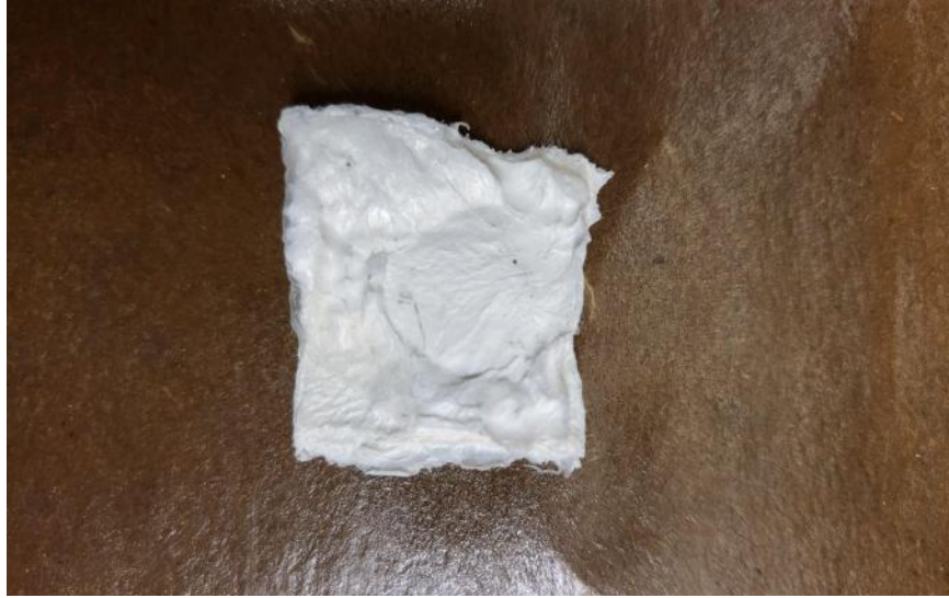
Figure 57. A 2.5 cm x 2.5 cm piece of liquid nitrogen frozen and freeze dried BC.
