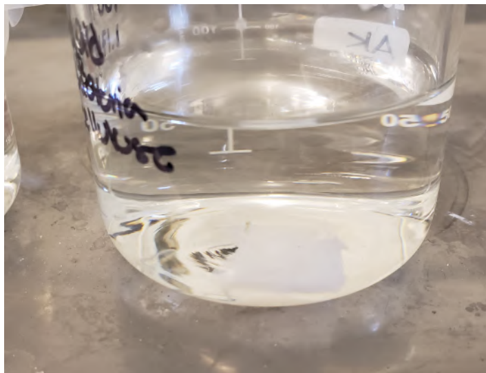
Figure 39. A piece of BC hydrogel submerged in 100 mL of 0.2M HCl. 1 week later.
