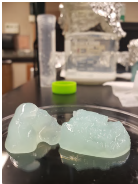
Figure 29. CNF hydrogel created after adding \text{Cu}(\text{NO}_3)_3 and waiting for 24 hours to completely react. Note that the solution was not agitated or mixed for hydrogel to form.
