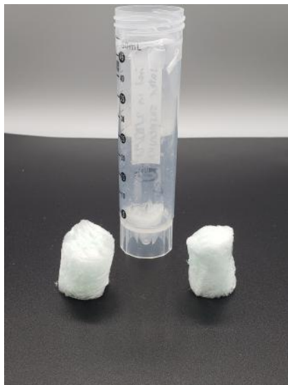
Figure 26. Hydroxyethyl cellulose hydrogel frozen in freezer then freeze dried.
