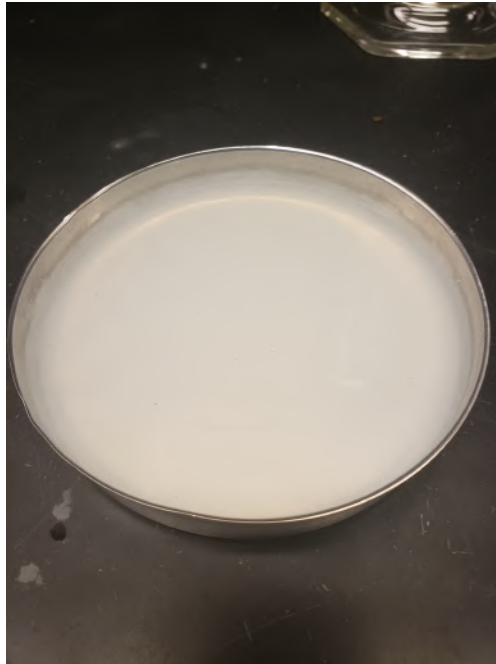
Figure 54. BC smashed with a house blender and mixed with HTO in an aluminum casting pan before oven drying at 60° C for 24 hours.
