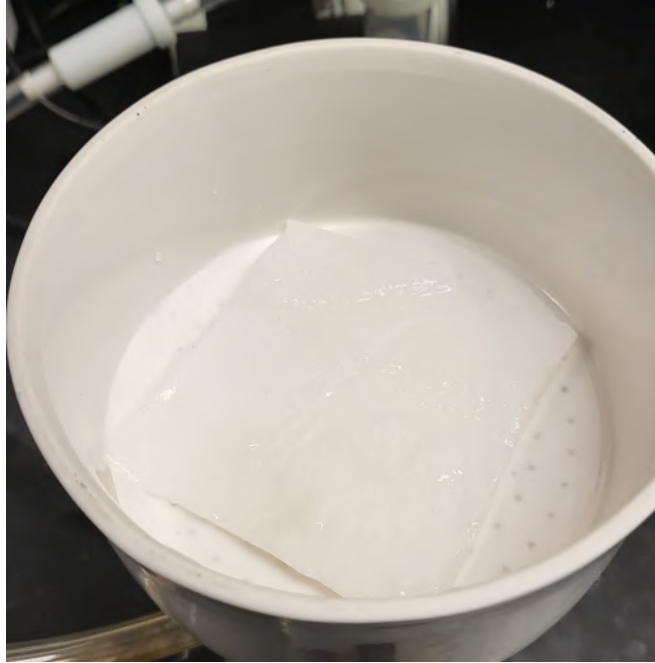
Figure 62. Overview of 8 cm x 8 cm of BC hydrogel placed in a funnel with a piece of 2.5 micron filter paper between them. Note that the hydrogel does not completely cover the funnel.
