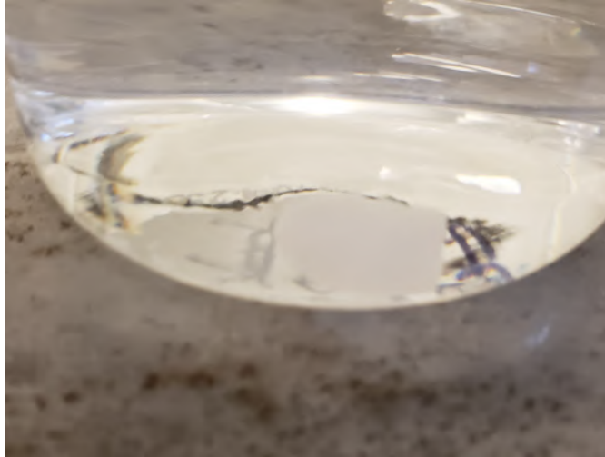
Figure 37. A piece of CNF hydrogel submerged in 100 mL of 0.2M HCl. 1 week later.
