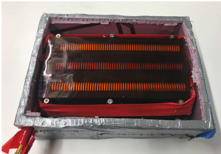
Figure 5.8: Power supply consisting of 400 cell-coin batteries of 3.2 Volts and 90 mA-hr each, connected in series, resulting in a total energy of 115 W-hr.
