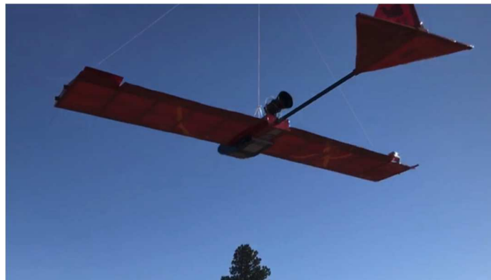
Figure 5.11: ELEPHANT 2A being launched using a high altitude burst balloon.
