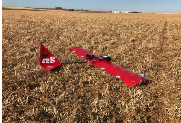
Figure 5.16: ELEPHANT 2B after landing. The aircraft was found on a corn field, with no major damage to the structure.
