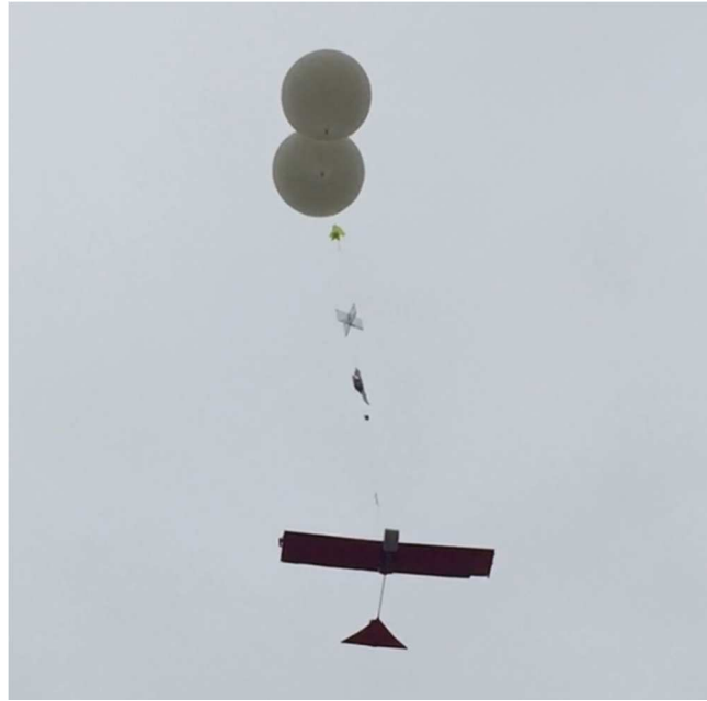
Figure 5.20: ELePHANT 3B launch. In order to extend the flying time, the aircraft was launched using two balloons, filled with lower amount of gas.
