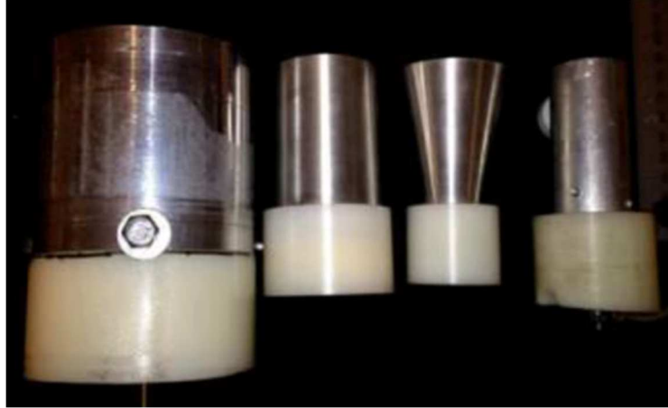
Figure 1.5: Early concepts of the Air-Breathing Pulsed Plasma Thruster developed at the Advanced Propulsion Laboratory (APL) in 2014 [12]. From left to right the diameter of the devices are 7.6, 5, 2.5-5, and 2.5 cm. All of the four concepts were 8 cm in length.
