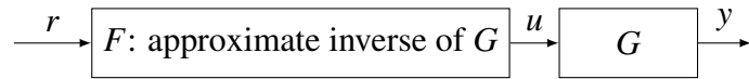
Figure 7.2: Block diagram to illustrate the goal of the model inversion design. Note that F can be implemented as a feedback/feedforward controller.
