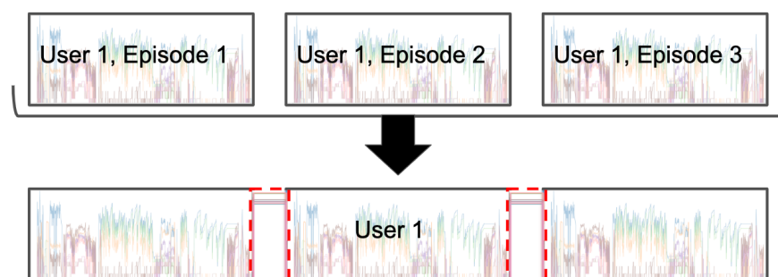
(a) The action series for a user's multiple sessions are combined into a single series with arbitrary noise (highlighted in dashed red) in between.
