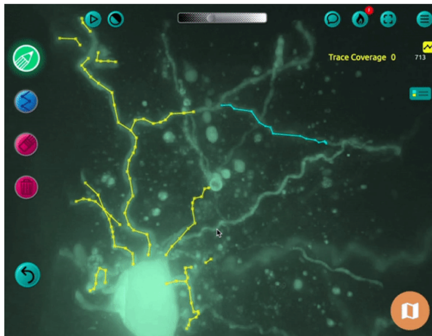
Figure 3.2: This figure shows the Mozak interface. The white lines and shapes are the neuron image being traced. The cyan line is the user's trace, while the yellow lines are the current consensus. Available tools are shown along the left side and buttons for altering the view and accessing the menu run along the top.
