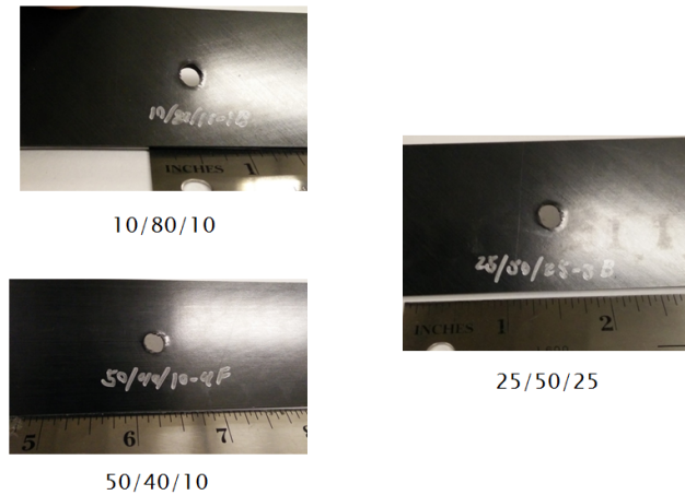
Figure 6.5: Delaminations observed on back side of received specimens
