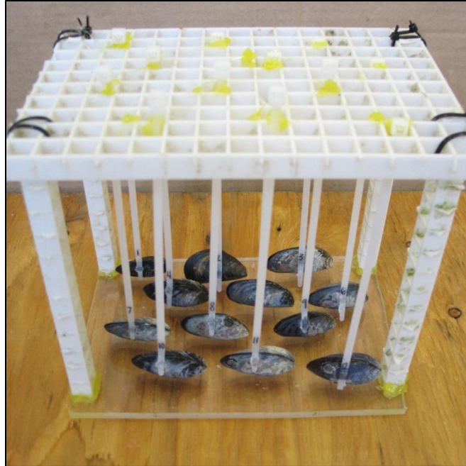
Fig. 3: Mussel rack design. Constructed with acrylic sheeting, plastic egg crate material, and hot melt adhesive, the mussel rack held 12 randomly chosen active mussels that were evenly spaced with anterior ends facing downstream to create a mussel “bed”. Mussels were attached to thin plastic rods with cyanoacrylate and suspended 6.5 mm above the acrylic sheet bottom.
