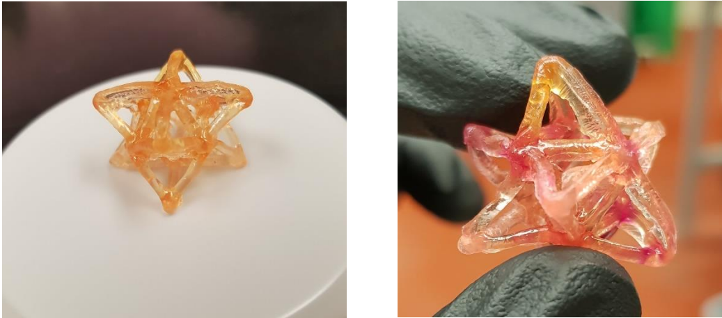
Figure 3.3 Left: Octet truss unit cell printed with HEA/BA 35/65 system; Right: Compressed octet truss unit cell.
