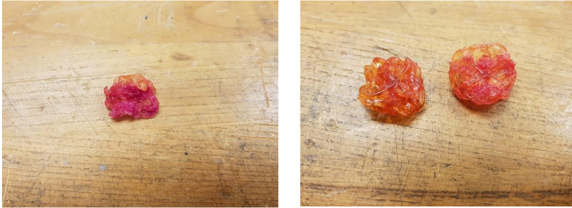
Figure 3.5 Left: Compressed octet truss unit cell printed with HEA/BA 35/65 system to near 100% strain; Right: Compressed octet truss unit cell printed with HEA/BA 65/35 system (left) and HEA/BA 80/20 system (right) to near 100% strain.
