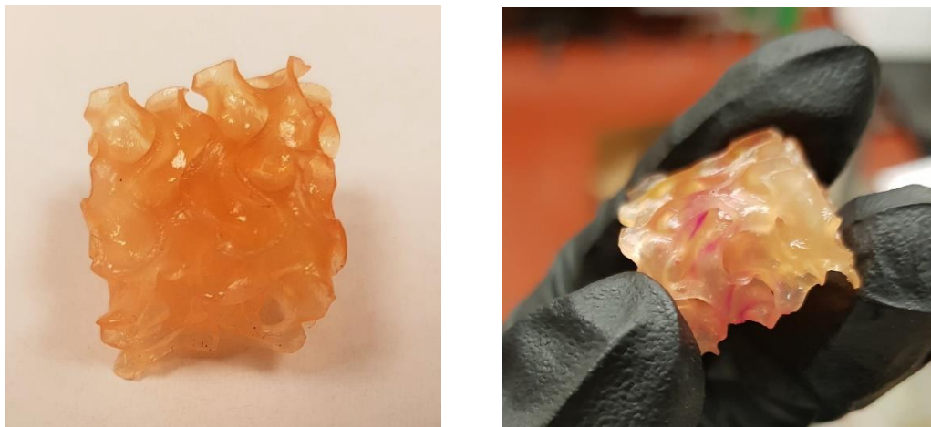
Figure 3.4 Left: Gyroid lattice printed with HEA/BA 35/65 system; Right: Compressed gyroid lattice.
