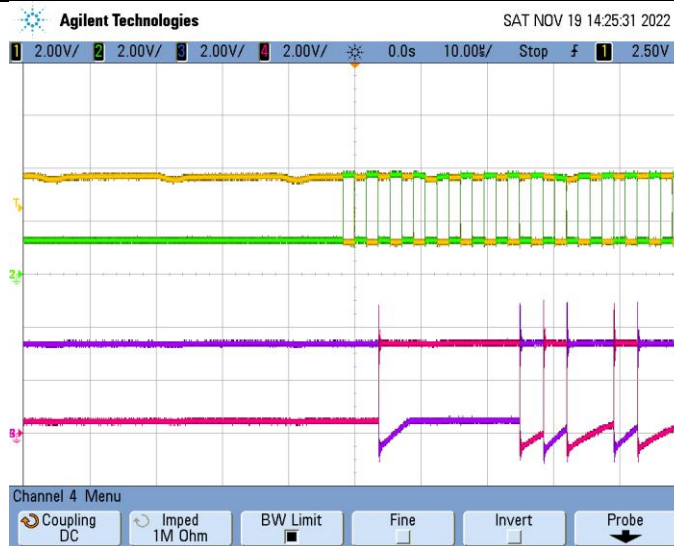
MA+, MA- (top) and SLO+, SLO- (bottom) on same oscilloscope capture.
