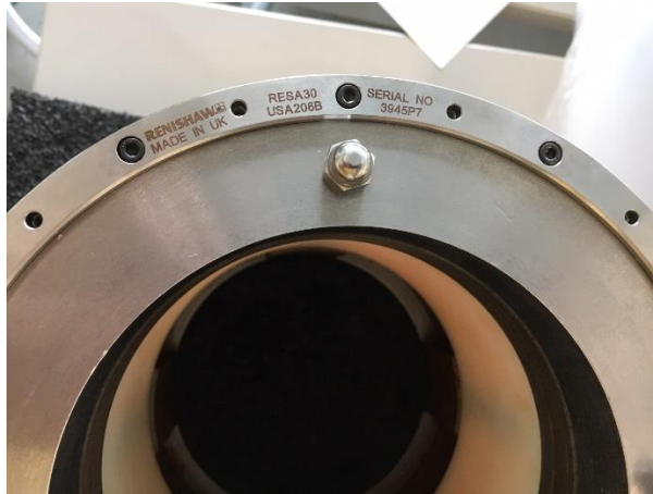
Figure 9.4 RESA30SA206B Rotary (Angle) Ring Part Number
