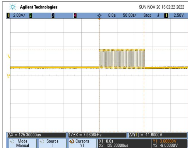
DB9 Connector Pin 3 (MA-). Shows MA- is complement of MA+, as expected.
