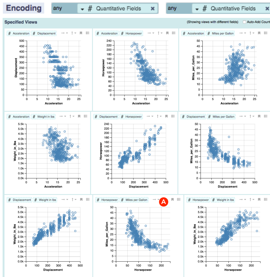
Figure 7.3: Dropping two quantitative field wildcards onto the wildcard shelves . Voyager 2 automatically chooses encodings, producing scatterplots that show bivariate relationships between all quantitative fields.
