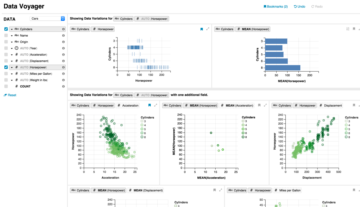
Figure 5.1: Voyager: a recommendation-powered visualization browser. The schema panel (left) lists data fields selectable by users. The main gallery (right) presents suggested visualizations of different field subsets and transformations in two sections. The exact match section on the top contains charts with all and only the selected fields. The suggestion section on the bottom contains charts with all selected fields and one extra field to encourage further exploration.
