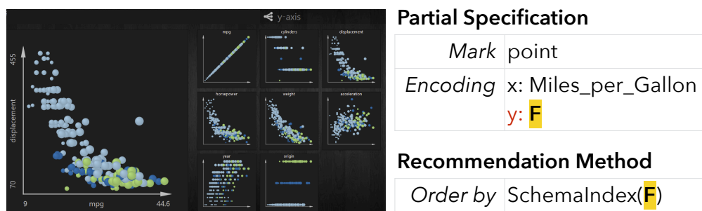
Figure 6.4: The Small Multiples Large Singles system [137] when a user chooses to enumerate the field on y-axis, expressed as a CompassQL query.
