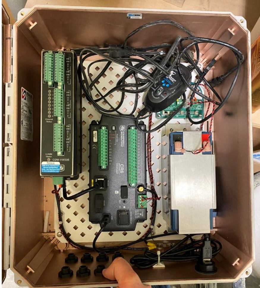
Figure 26. CR6 Datalogger and VW interface in enclosure
