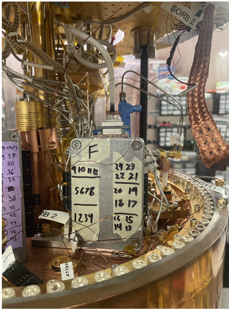
Figure 2.19: The newly designed breakout box for Cable F mounted on top of the cavity next to the breakout box for Cable E (left edge of the image). The connectors for temperature sensors can be seen on the left hand side of the breakout box and there are 3 spares. Cable F is shown plugged into the top of the box.
