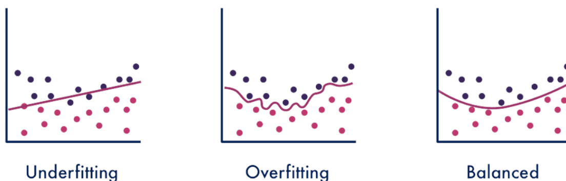
Figure 2.3: Optimal model fitting [6]. The under-fit curve (left) lacks the complexity needed to model the data, which results in both high training and test error. The overfit curve (middle) matches the existing data points too closely, so while the error on the training set is low, any new unseen data points are likely to have high error rates. The balanced fit (right), strikes the balance between the two extremes, which is what we hope to obtain in model fitting.
