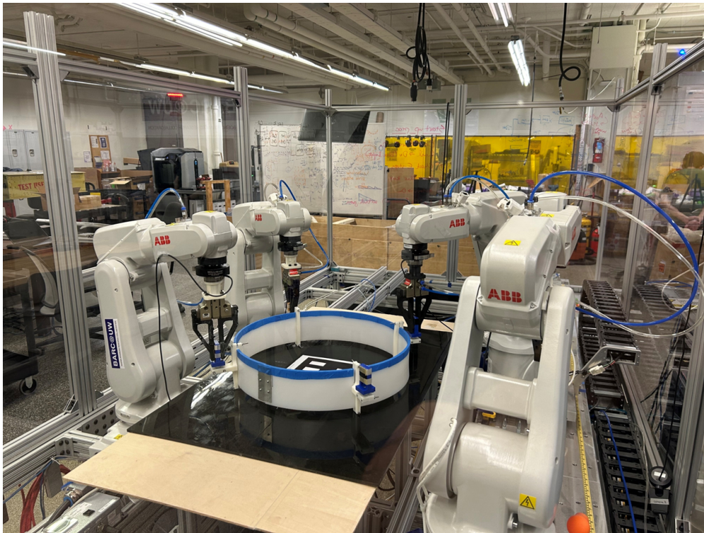
Fig. 6.1 | Robotic validation platform for discrepancy model verification showing flexible structure with robotic actuators
