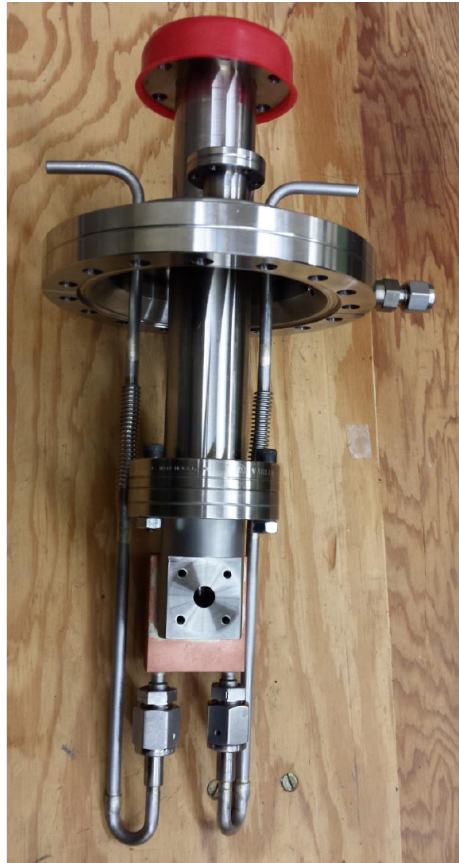
Figure 2.12: The latest target design eliminated areas of failure and is more suited to long-time, high-intensity use than previous iterations.
