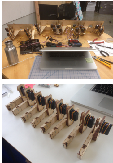
The final set of arms coming together, being tested, bug fixing the electronics and code, and installed on the display panel.
