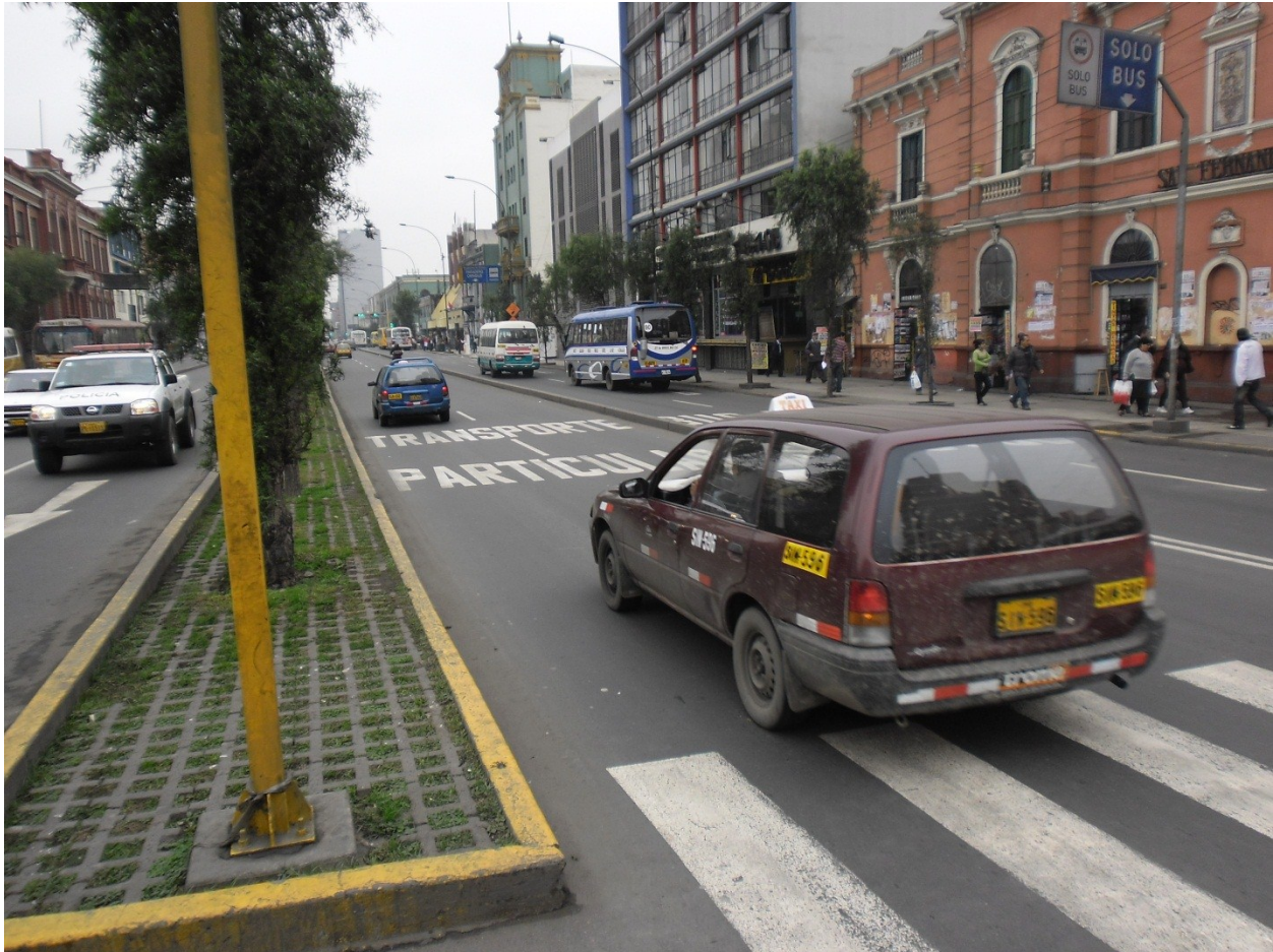
Figure 5. Curb-side or exterior type bus lanes (far right lanes) with private/mixed vehicle traffic in the median lanes.
