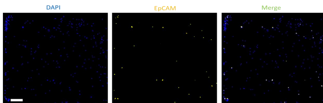
Figure 2.5 Fluorescent images of collected cells after sorting with a 2-stage 3 cm-channel chip. DAPI (blue) channel showed cell nuclei of collected cells and PE-EpCAM (yellow) channel showed MCF-7 cells. The scale bar is 500 \mu\text{m} .
