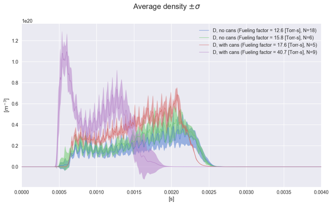
Figure C.3: Comparison of chord-integrated electron density with and without passive pumping (“cans”) in deuterium discharges. In this case the opposite trend is observed.
