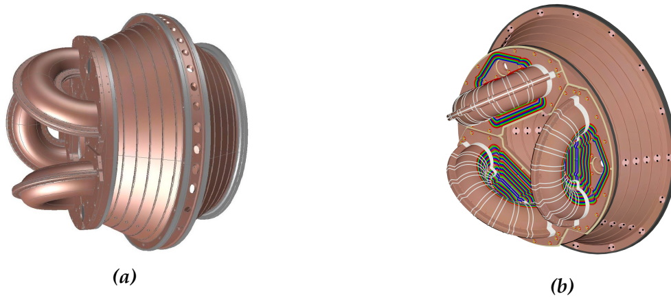
Figure 2.3: (a) The bare HIT-SI3 injector and confinement volume structure. The three copper half-tori (left) inject plasma, energy, and helicity into the main chamber. The gapped midplane allows for diagnostic access. (b) “Flux” coils shown in white generate magnetic field along which current is induced by transformer action of the “voltage” coils shown in red, green, and blue.
