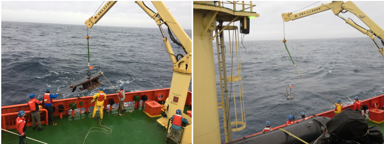
Figure 2: Wave Glider launch via crane (left) and release (right) from the R/V Laurence M. Gould in a calm region protected by the South Shetland Islands.
