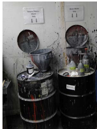
Figure 15 Waste drums with funnels to capture waterborne waste
