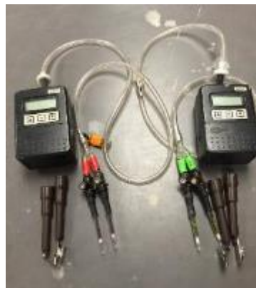
Figure 4 Two-pump setup Red tape: manifold #1 Green tape: manifold #2
