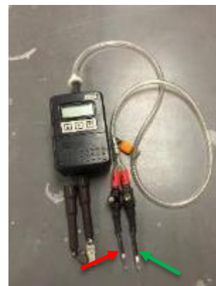
Figure 5 One-pump setup Red arrow: O90 sorbent tube Green arrow: CSC sorbent tube
