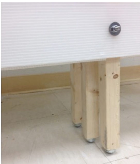
Figure 40 - Single ball caster for each panel's leg
