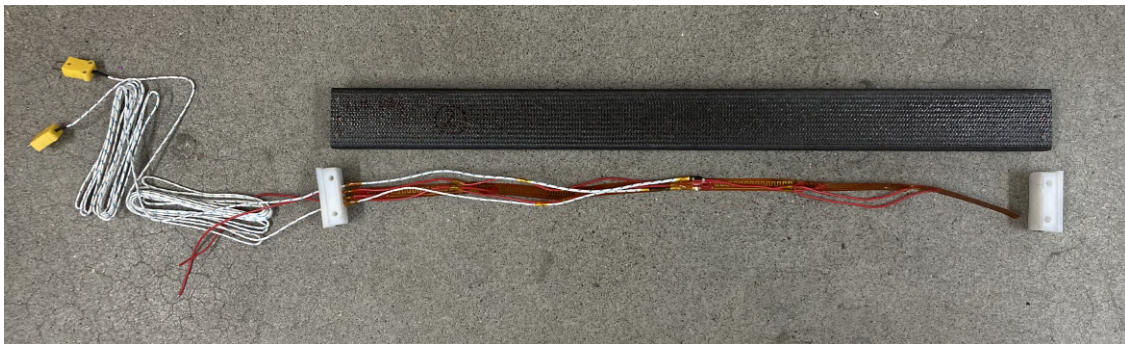
Figure 3.13: A specimen before assembly with heater wires in red and thermocouple wires in white.
