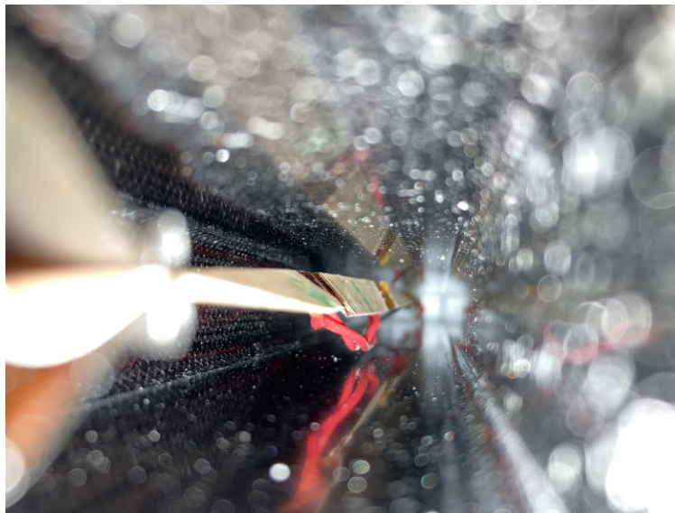
Figure 3.16: View of the heater strand inside the specimen before being filled with multiphase material. It can be seen here that the heater strand was centered well in the specimen but due to its flexibility was not kept perfectly oriented.
