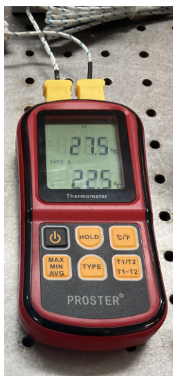
Figure 3.7: Thermocouple thermometer used to read the temperature. Only one thermocouple was used for temperature reading in these experiments. In this case, the second is to compare with room temperature.
