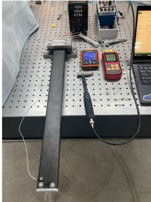
Figure 3.14: Experimental modal test setup with instrumentation in cantilever boundary conditions. The accelerometer can be seen attached at the tip of the beam. Shown to the side are the DC power supply, DAQ, thermal imaging camera, thermocouple thermometer, modal hammer, and computer.
