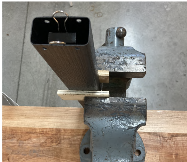
Figure 3.17: Vice holding the prepared carbon fiber specimen set up to have the uncured silicone poured in the top opening. A binder clip is shown holding the end of the heater strand in order to make sure the heater was centered properly in the beam as the mixture was poured.
