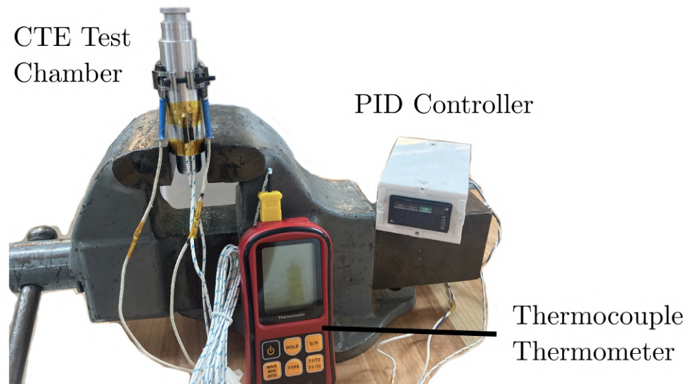
Figure 3.3: CTE testing chamber clamped in a vise without insulation for demonstration purposes. PID controller and thermocouple thermometer connected and shown to the side.
