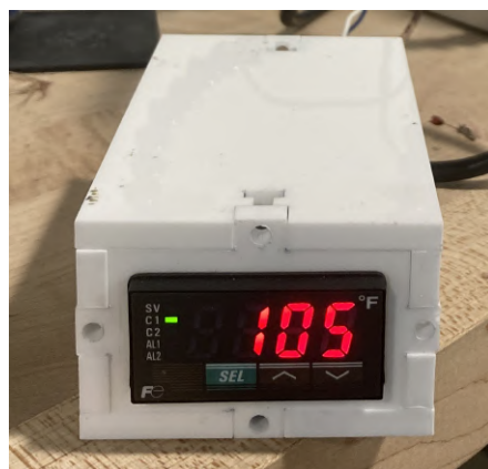
Figure 3.6: Proportional-integral-derivative (PID) controller used for controlling the heater in CTE experiments. This device was set up to use thermocouple temperature readings to heat each specimen at the same linear rate.
