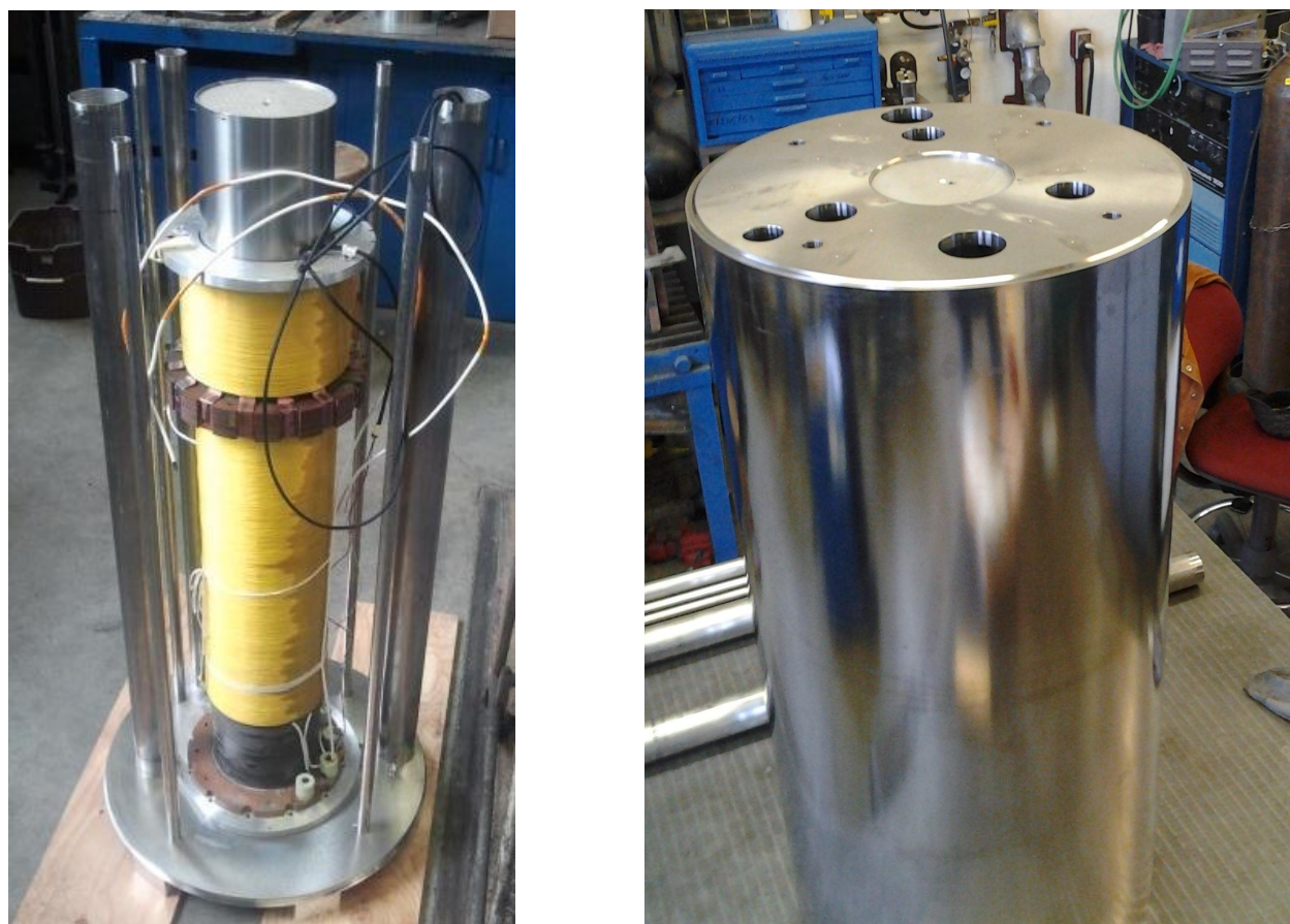
Figure 3.16: At left, a picture of the bucking coil being installed within the reservoir. The bucking coil fits around the reservoir bore tube and bolts to the reservoir bottom. At right, a picture of the reservoir as it is being machined. The large central bore is to accommodate the squidadel with the MSA and other electronics. The surrounding through tubes run various plumbing pipes and wires that go from warmer stages down the Cold space.
