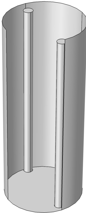
Figure 4.3: COMSOL cavity model. The top endplate and one quarter of the barrel are hidden from view. The cavity itself is represented as a right circular cylinder, as are the two tuning rods. The rods have a 1/2" gap to the top and bottom cavity endplates.
