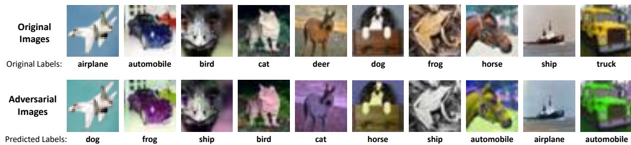
Figure 1.3: Samples of CIFAR10 original images (top) and semantic adversarial examples (bottom) on VGG16 network. Adversarial images are generated by converting original images into the HSV color space and randomly shifting the Hue and Saturation components, while keeping Value the same. All images in first row are correctly classified by the model.
