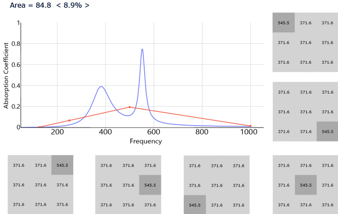
Figure 29: Different arrangements between identical resonators and one resonator with a larger neck radius produce the same absorption graph
