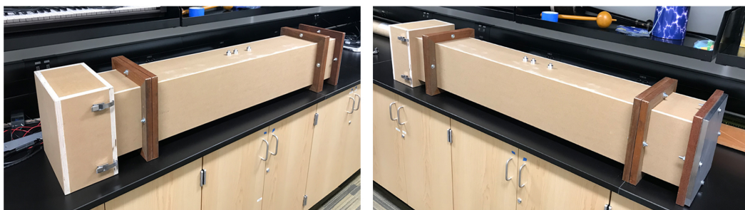
Figure 96: View of the completed impedance tube setup
