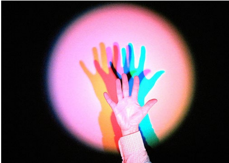
Figure 1-22. Subtractive color resulting in colored shadows. Photo courtesy of The Physics Classroom
