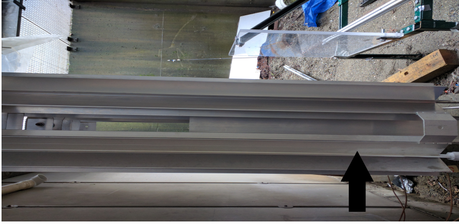
(b) Frost growth at the end of test.
