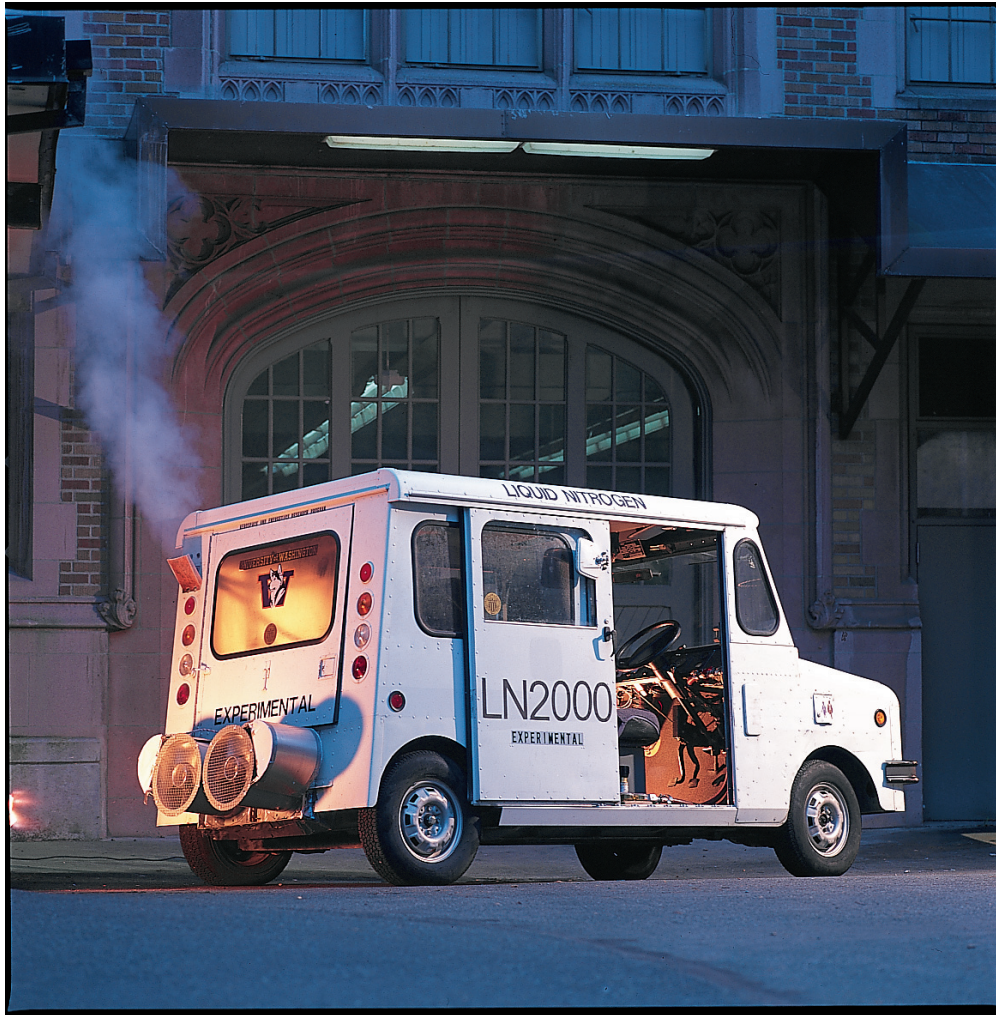
Figure 1.2: Liquid nitrogen powered vehicle, designed and built by previous UW students. The LN2000 was used to study the feasibility of a zero emission vehicle concept [5].
