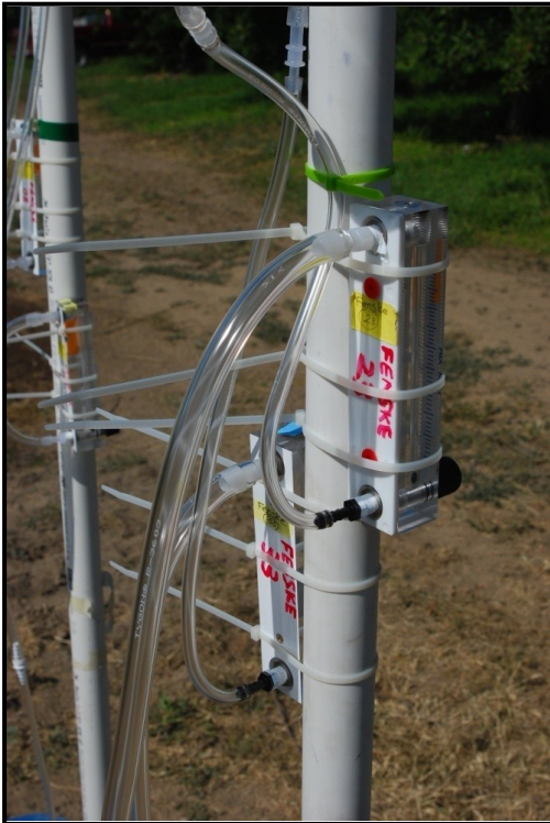
Figure 8.1/ Connected rotameters to sample mast.
