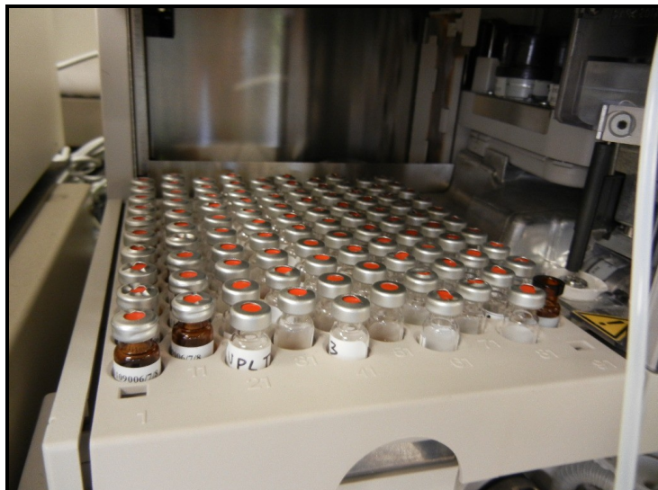
Figure 8.10 Loading LC-MS extraction vials for analysis.
