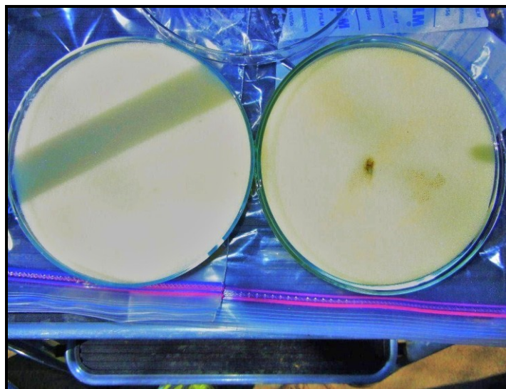
Figure 8.8. Placing PUF disk in the glass petri dish. The disk on the left is a field blank and the disk on the right was deployed.
