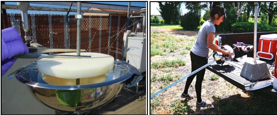
Figure 8.5. Placing PUF Disk inside PUF-PAS housing.
