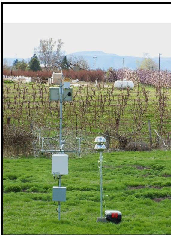
Figure 5.2/ Outdoor Testing Sites of PUF-PAS devices. The figure on the left is a testing site in Seattle, WA. The figure on the right is in Yakima Valley, WA. The device is located near an orchard and a WSU AgWeatherNet Meteorological Station.
