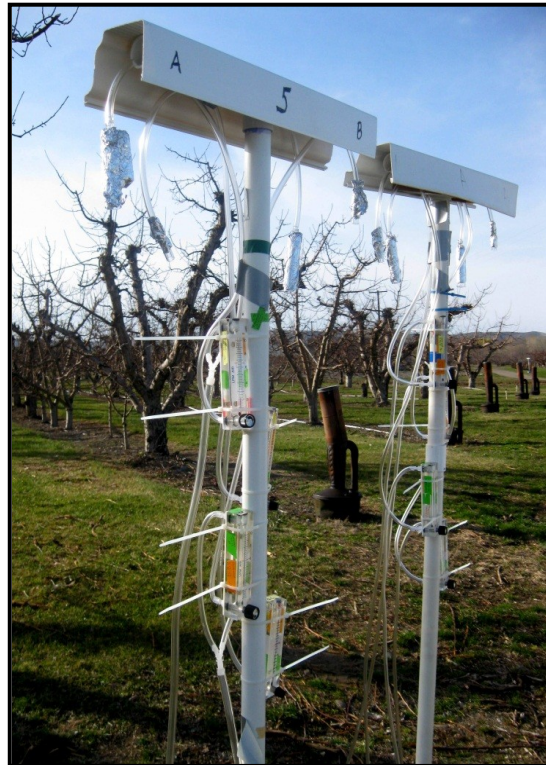
Figure 8.2/ Hanging OVS/PUF Tubes.
