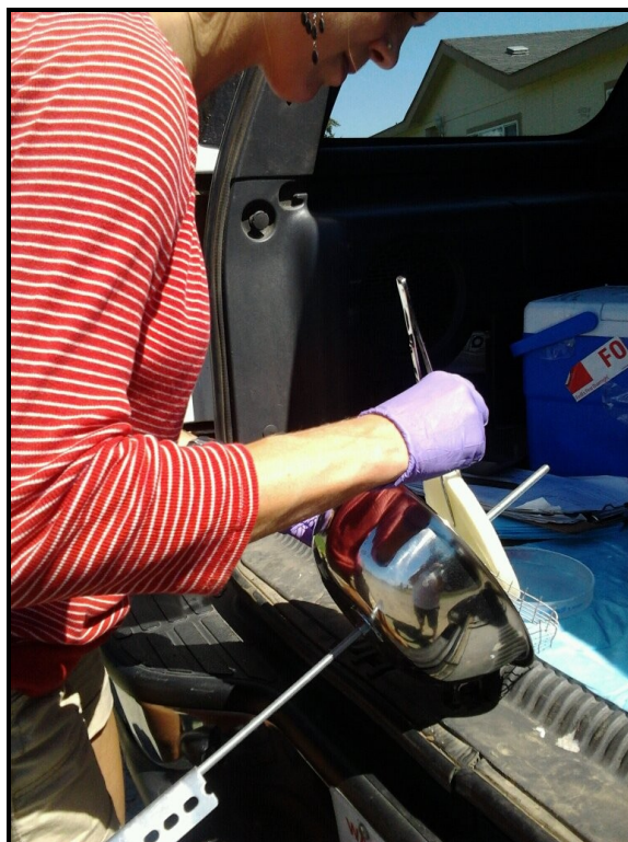
Figure 8.7. Removing PUF disk from the sampling device.
