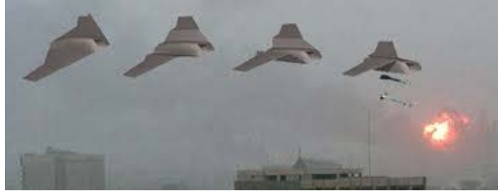
Figure 1-2: Lockheed Martin “Z-Wing” morphing concept vehicle
