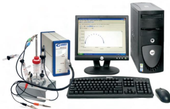
Figure 4.2. Conventional setup used to perform cyclic voltammetry
