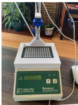
Figure 3.4. Peltier hot/cold plate used to freeze and/or heat the samples on the well plate
