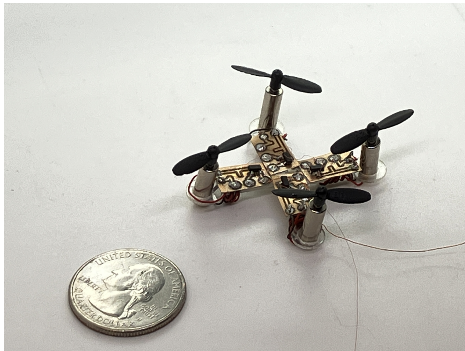
Figure 4.4: The acrylic version of the chassis used to evaluate motor and motor controller positioning.
