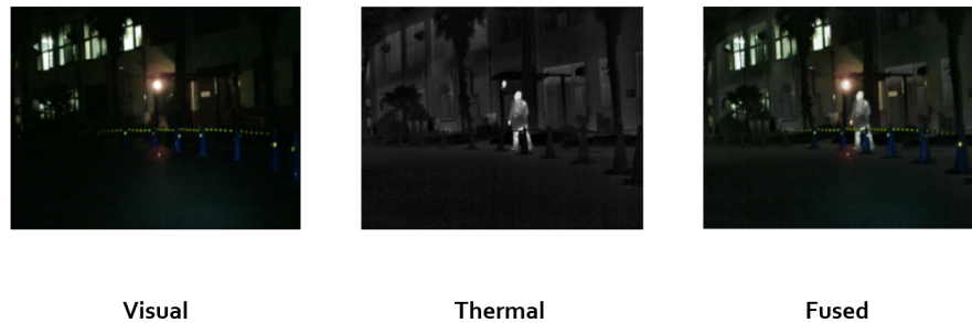
Figure 1.4: In the provided illustration, we observe the fusion of a visual image (on the left) and a thermal image (in the middle), resulting in the fused image (on the right).
