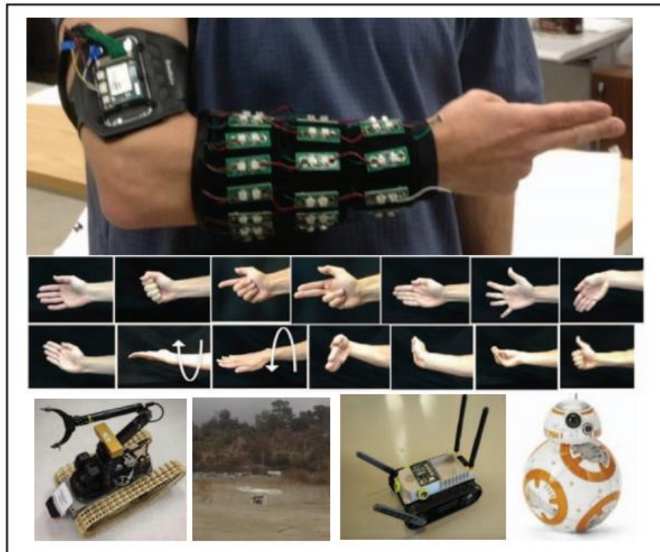
Figure 1.2 Wearable bio-sleeve for hand-free gesture control of robots [28].
