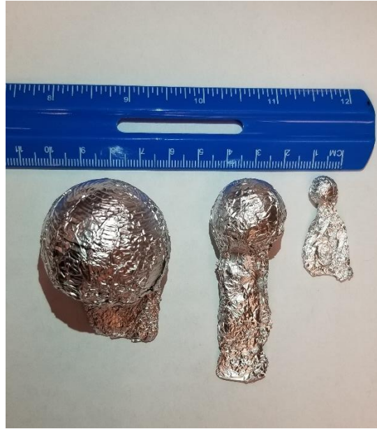
Figure 5.12 3D printed spheres (10, 25 and 40mm) covered with Al foil.
