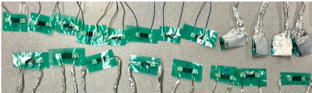
Figure 5.4 (a) Picture of CPC eye tracking sensor. (b) 20 fabricated CPC eye tracking sensors that can work properly. The folded sensor is a cantilever-shaped sensor.
