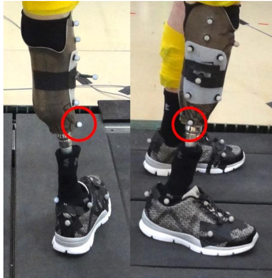
Figure 3-4. Static trial images showing the placement of the pylon marker. This marker is later used in scaling to separately scale the residual limb and pylon segments.
