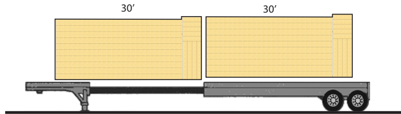
Flat pack classroom: Two classrooms with one 70' trailer (max length) flatbed trip
