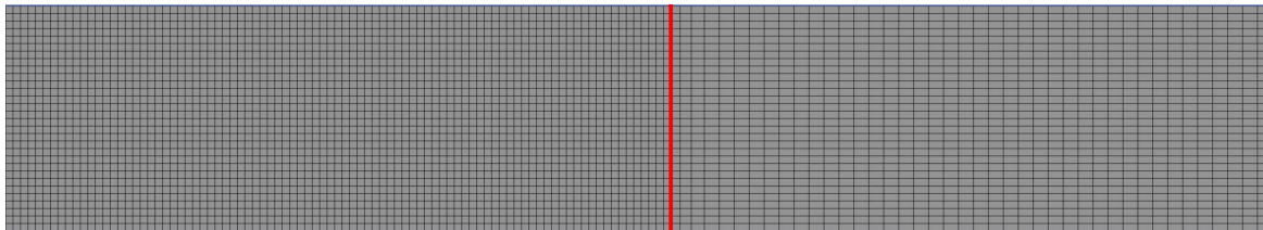
Figure 5.7: Sod mesh example with 0.5 mm elements in the driven (left) and 1 mm elements in the driver (right). The diaphragm is represented by the red line. The total mesh has 45,060 elements, 46,593 nodes, a minimum orthogonal quality of 1, a minimum element quality of 0.799, and a maximum skewness of 4.27e-7 .
