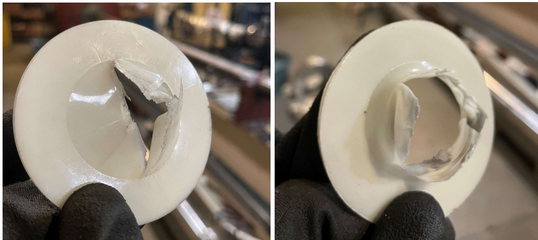
(a) Partially opened diaphragm.
