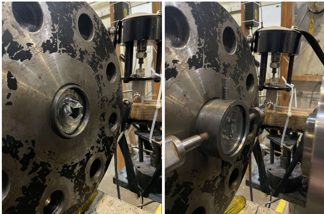
(a) Upstream driver diaphragm, post-shot. (b) Downstream driven diaphragm, pre-shot.
