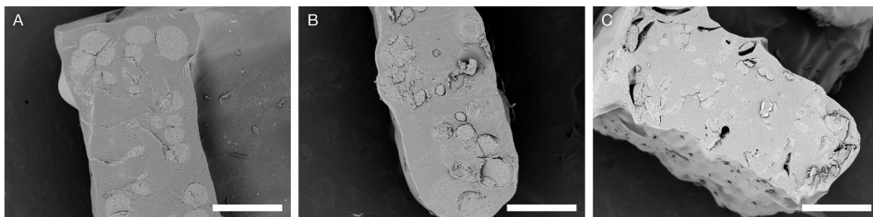
Figure D.S8. SEM micrographs of LMs after 72 h incubation. F127-DMA (A), F127-BUM (B), PGE-DMA (C).
