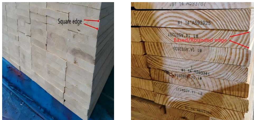
Figure 4.1. Comparison of lumber edge profiles observed during field visits: (left) square-edged lumber observed at a European sawmill and (right) eased-edge lumber observed at a North American CLT manufacturing facility.
