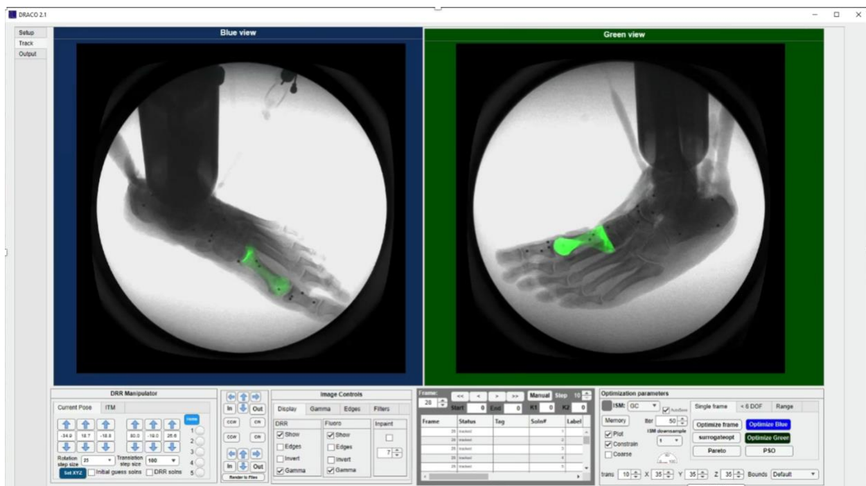
Figure 1: Graphical user interface of the DRACO software. The stereo fluoroscopy views are displayed with the DRR of the currently selected bone overlaid. Translation and rotation manipulators allow the user to set the initial guess pose of the bone prior to optimization. The user also has control of various image processing and edge detection parameters to enhance and aid the alignment via the optimizer.
