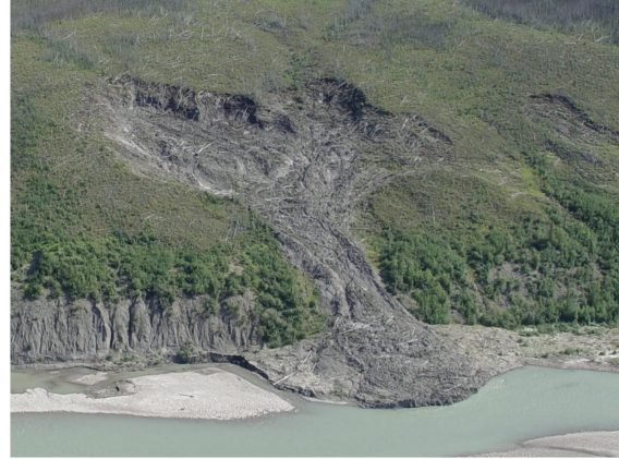
Figure 2.7 Simplified diagram (left) and an example Flow Slide. Source often region similar to lateral spreads, in agricultural or otherwise developed land, large highly disrupted displacements with some evidence of fluidization or semi-fluid like flow. Figure from Highland and Bobrowsky (2008), based on Cruden and Varnes (1996), photograph by Marten Geertsema.
