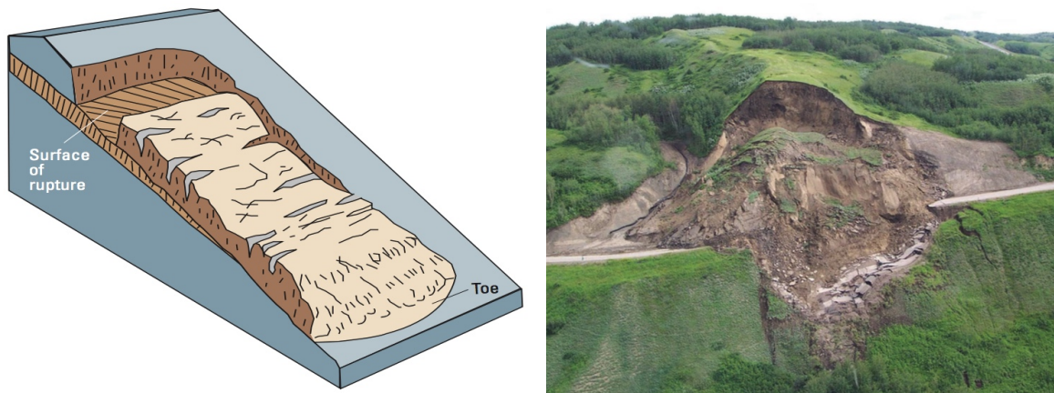
Figure 2.6 Simplified diagram (left) and an example Debris Slide. Often high in the landscape along undeveloped, steep, hillslopes. Shallow failure surfaces with highly displaced and disorganized mobilized material. Figure from Highland and Bobrowsky (2008), based on Cruden and Varnes (1996), photograph by Réjean Couture.
