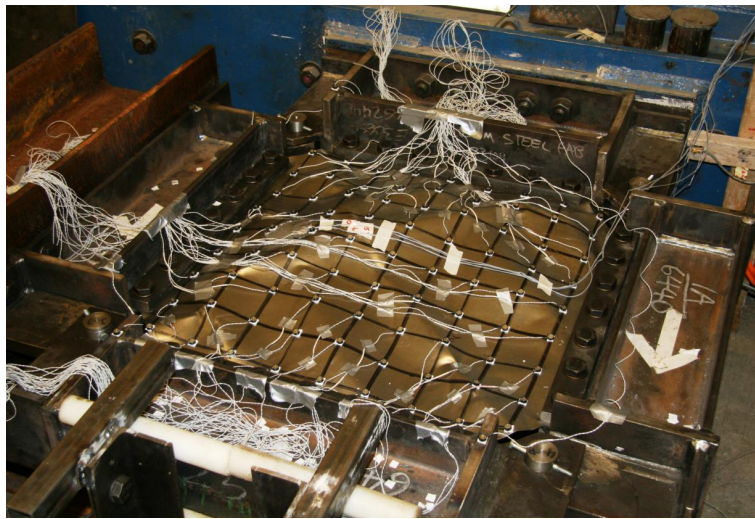
Figure 5.10: Test # 1-18 residual web plate deformation at completion of test.
