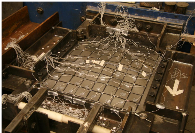
Figure 5.9: Test # 1-18 residual web plate deformation at end of cycle # 8.
