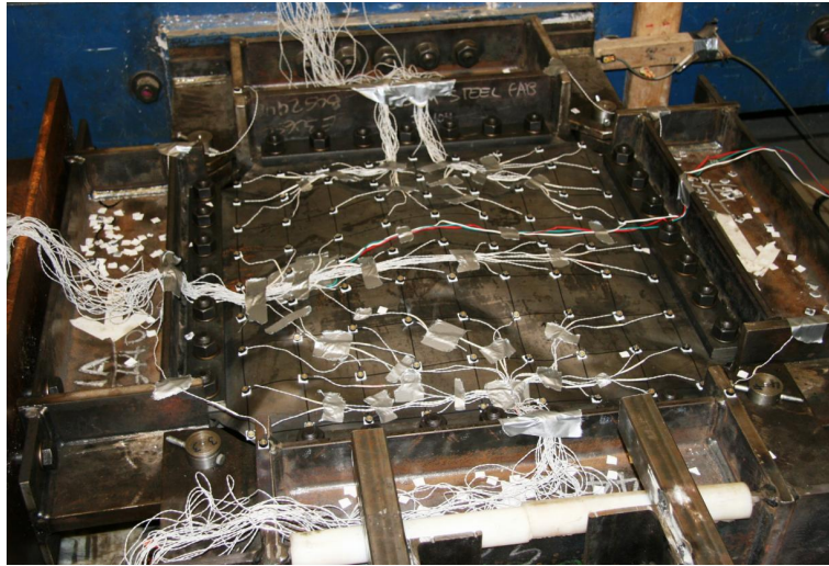
Figure 5.21: Test # 1-16 web plate residual deformation after cycle # 18.
