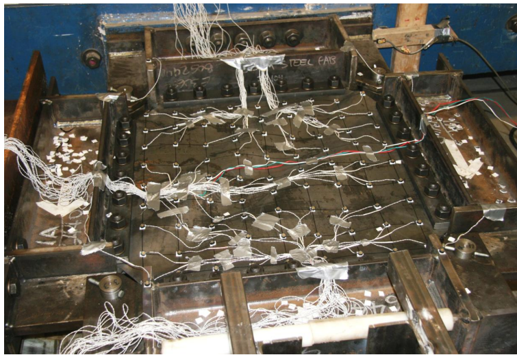
Figure 5.19: Test # 1-16 web plate deformation at peak of cycle # 18 pull stroke.
