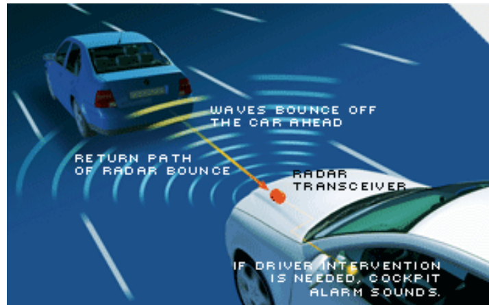
Figure 1. ACC control system
