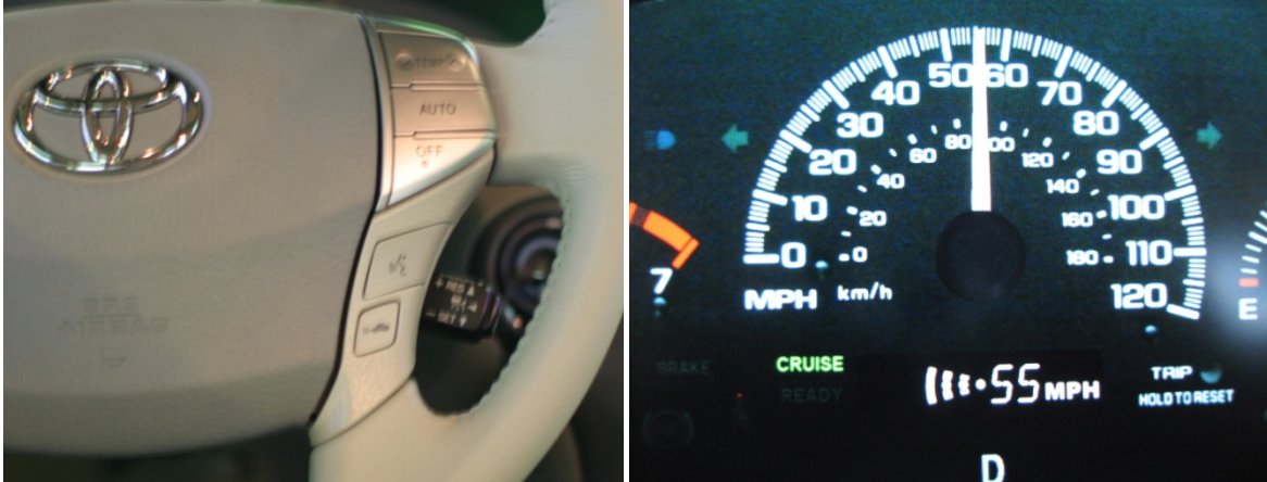
Figure 16. ACC controls (left) and display (right) in the motion-based simulator
