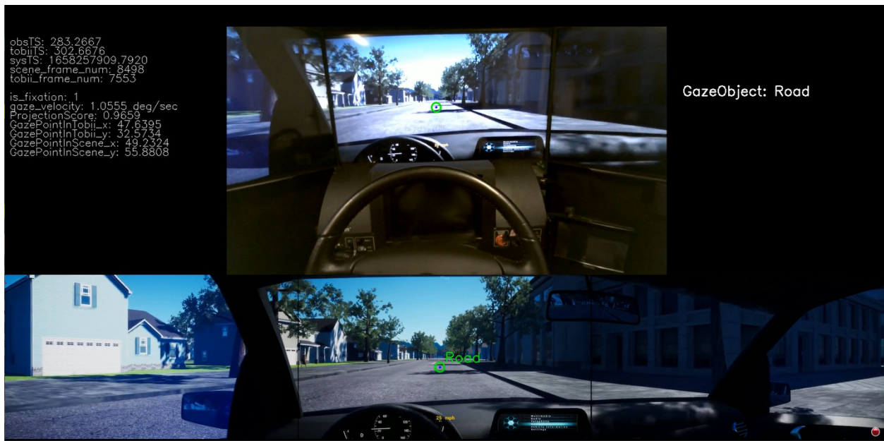
Figure 4.1: Tobii eye tracker was used to collect driver eye-gaze data. The top image is eye tracker recording from driver and the bottom image is the three screens of driving simulator.
